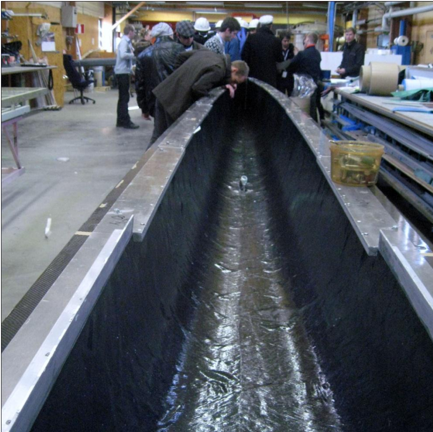
Composite hull of a catamaran
