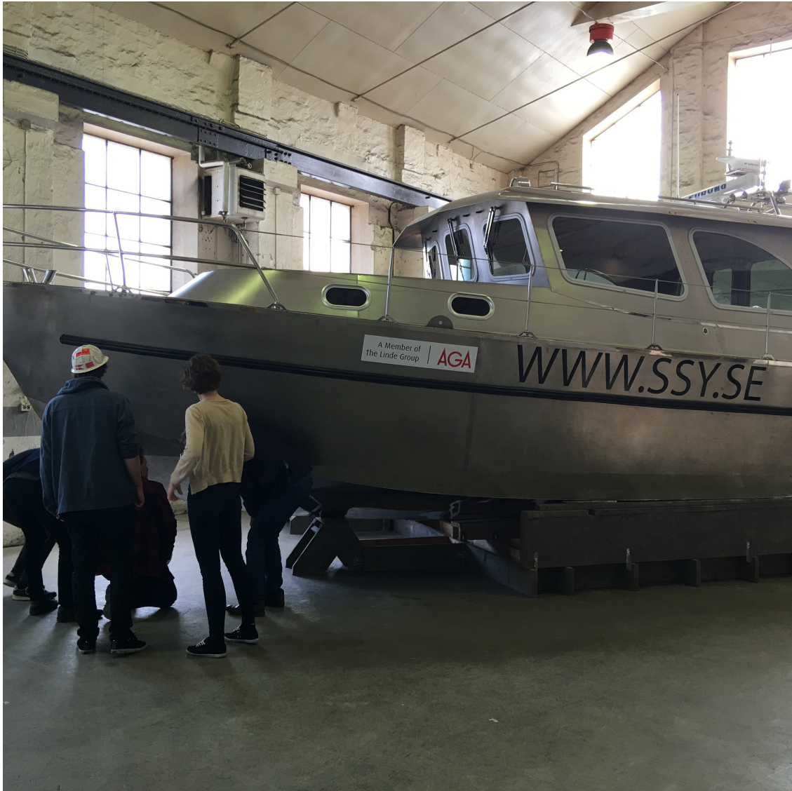
Figure 7: The first prototype made entirely out of stainless steel.
