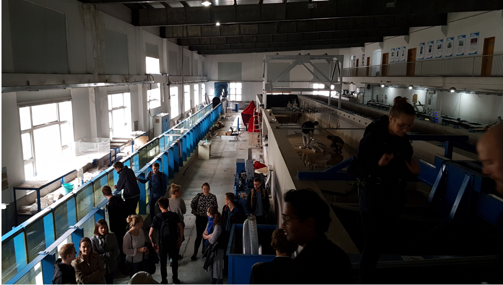
Figure 12: Overview of the tanks in the Laboratory of Fluid Dynamics. From right to left: Wave tank, tsunami tank and a varying density tank.
