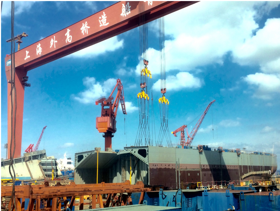
Figure 7: SWS - a megablock being lifted into place.
