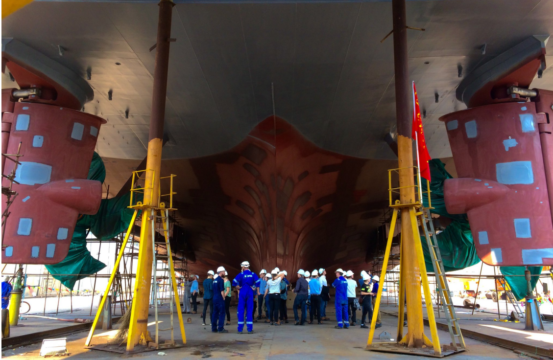
Figure 19: The group standing underneath the hull of the almost complete vessel in the dry dock. The propellers, with green covers, and the rudder can be seen in the sides of the picture.
