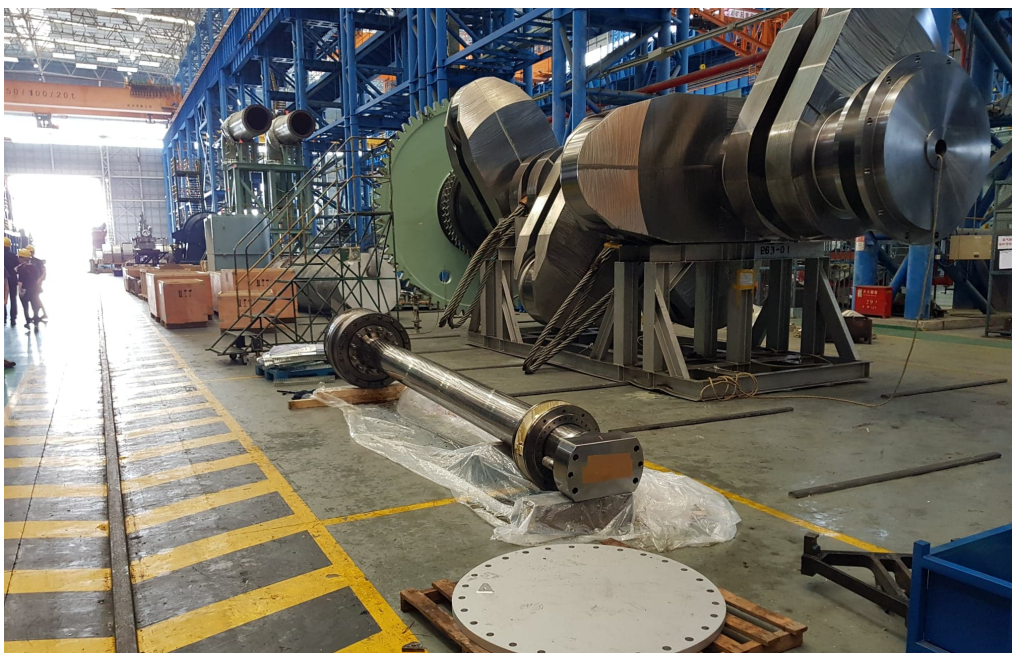
Figure 24: Crankshaft and piston for marine diesel engine.
